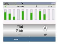
When using your ViaMichelin Navigation X-970 for the first time, we recommend you to do so in an open space in order to ensure the best possible satellite reception. Activating the GPS system for the first time can take several minutes, depending on the surroundings and the quality of the GPS signals.
